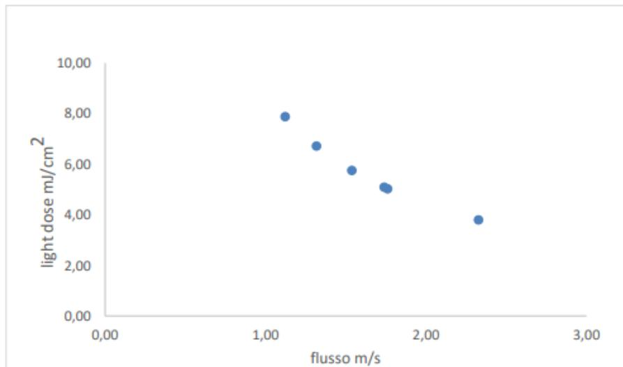
Figure 5. Trend of radiant energy density related to the speed of air inlet.
