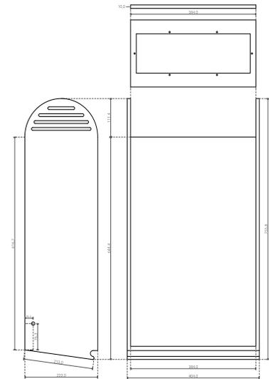
Figure 2 – dimension of the irradiation chamber
